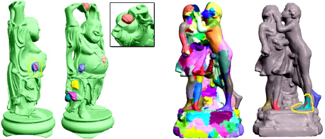
Fig. 9. Self-shape matching. Left: a flower is cut out using our interactive tool. Middle left: the other five similar salient geometric features on the Buddha model are retrieved using the partial matching operator. Middle right: aggregates at level 7. Right: given one foot extracted using our interactive tool, three other feet are automatically retrieved
