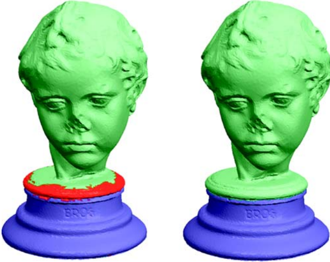
Fig. 6. Left: the fuzzy region (in red) during boundary optimization of a salient feature (in blue). Right: the final optimized feature boundary
